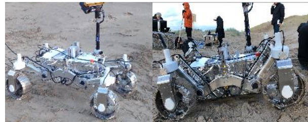
Figure 4: Left - nominal chassis height for navigation. Right: lowered chassis to perform drilling operation.
