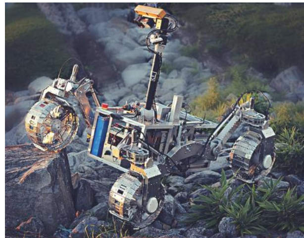
Figure 5: LUVMI rover – highlighting the benefit of the passive rocker-bogie for obstacle clearance
